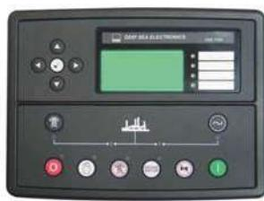
The **DSE7310** is an Automatic Start ControlModule and the DSE7320 is an AutoMains (Utility) Failure ControlModule. Both modules have been designed to start and stop diesel and gas generating sets that include electronic and non-electronic engines.
